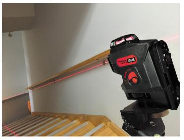
Unit featured is 3D3XR in manual mode. Also pictured is an optional iet68 elevating tripod and optional GD12 grade dial plate; a camera style tripod with pan and tilt will provide a similar result.
