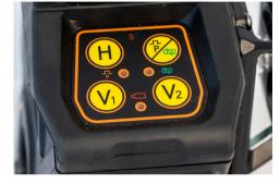
Next select the lasers press either the "H" Horizontal button or "V" Vertical buttons. To power down the laser level simply re-lock the pendulum by switching it to the "OFF" Position.
