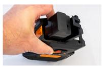
To charge this battery pack simply insert the charger cable into the charging socket on the Li-ion battery pack itself. Note; the socket on the laser level is for service use and the supplied charger does not fit this...
